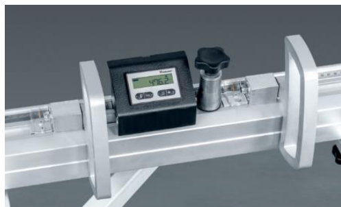
DDF: Digital read out on 1st flipper stop of CZ crosscut fence
