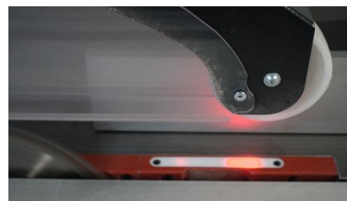
LED warning for functioning scoring blade
